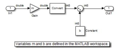
The  $\tt PreLoadFcn$  callback function defines m and b in the MATLAB workspace when you open the model:
