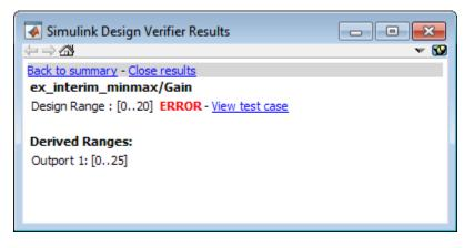
When the software detects an error, the analysis proceeds, but constrains the signal to the tightest intersection of the design range and the derived range, which for the Gain block output in this example is [0..20].
