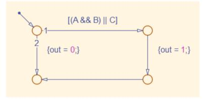
Given that A, B, and C are all separate inputs, there are five possible ways to evaluate the condition on the Stateflow transition, shown in the following table.
