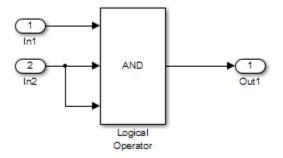
When the Simulink Design Verifier software analyzes this model for Condition Decision coverage, the analysis can only satisfy five of six objectives for the Logical Operator block inputs. The software cannot generate a test case when the third input to the Logical Operator block is false. If the second input is false, the third input is false, but the software ignores the third input due to the short-circuiting. If the second input is true, the third input is never false.
