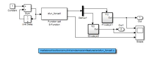
subsystems f1 subsys1 and f2 subsys2 on the first and second elements of the first output port.
