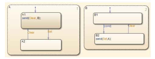
If you change the send function calls to use directed event broadcasts so that the Set and Clear events are broadcast directly to the states B1 and A1, respectively, the cyclic behavior disappears and the Simulink Design Verifier software can analyze the model.
