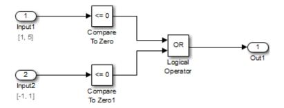
When you analyze this model using the Simulink Design Verifier software, the analysis uses the minimum and maximum values as constraints. The analysis produces the following results:
