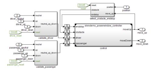
$The \verb| control Model block references the \verb| slvnvdemo_powerwindow_controller model.$
