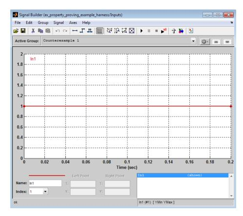
The input signal 1 causes the output of the Compare to Zero block to be 0. This counterexample violates the proof objective that specifies that the output of the Compare to Zero block be 1.
