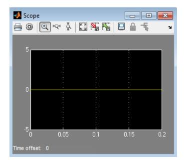
The Scope block displays the value of the signal output by the Compare To Zero block in your model. In this example, the Compare To Zero block returns 0 (false) throughout the simulation, which falsifies the proof objective that the output of the Compare to Zero block be 1 (true). The counterexample that the Signal Builder block supplies falsifies the proof objective.
