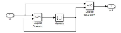
The persistent information in this model is limited to the Boolean value of the Memory block. The input to the model is a single Boolean value. The following table describes the complete behavior of the model, including the behavior that would result from an arbitrarily long sequence of inputs.
