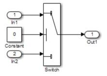
For this Switch block, the control input is always 0. If the **Criteria for passing first input** block parameter is  $u^2 \sim 0$ , the Switch block always passes the third input through to the output port. When you analyze this model, the Simulink Design Verifier software removes the Switch block from the model and does not report any test objectives for the Switch block.
