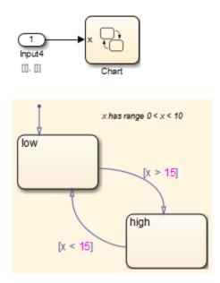
The value of x must fall between 0 and 10, so the transition condition [x > 15] is never true. The transition from low to high never occurs. Because the high state is never entered, the transition condition [x < 15] is never tested, and the transition from high to low never occurs; the chart is always in the low state.
