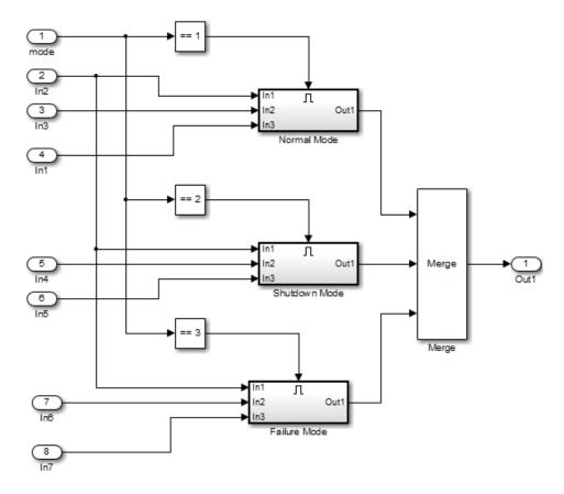
You can incrementally generate test cases for each subsystem by constraining the first input to a constant value before running an analysis. In this way, as you create test cases for each subsystem, the software ignores the complexity of the other two subsystems.
