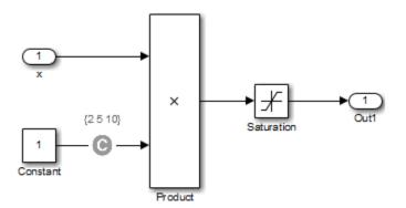
• When you work with large models that have many multiplication and division operations, you may find it easier to add constraints to all of the floating-point inputs rather than to identify the precise set of inputs that require constraints.
