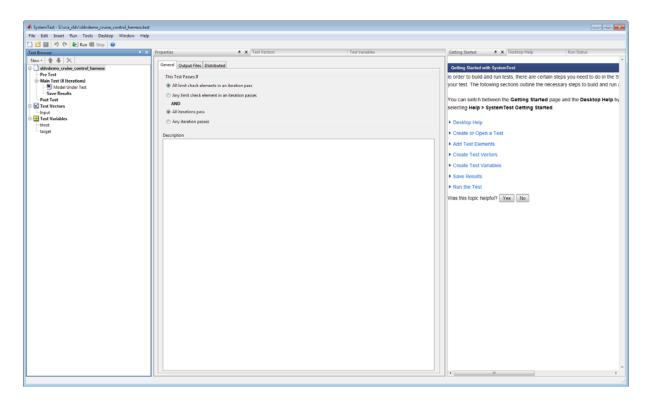
In the **Test Browser** pane, the 8 iterations in **Main Test (8 Iterations)** correspond to the 8 test cases that the Simulink Design Verifier software generates and describes in the Test Case Explanation block of the harness model.
