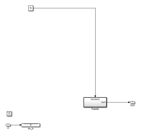
The new Inport block A writes into the data store, which is used by the subsystem Reader in the new model.
